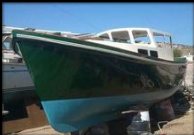
CW 25'-6" Bora showing typical classic high bow shape and canoe stern of the Colvic Watson design
