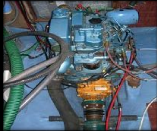
Typical 27.5 hp & 30hp engine bay CW 23'-6"
