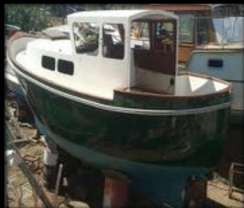
CW 25'-6" Bora showing typical classic high bow shape and canoe stern of the Colvic Watson design
