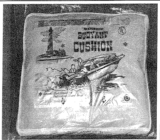
Fig. 8 Type II buoyant cushions are made to be thrown to people in the water. If you can squeeze air out of the cushion, it is faulty and should be replaced
