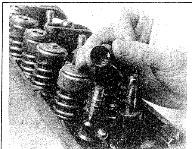
Fig. 147 Removing an umbrella/positive type seal
