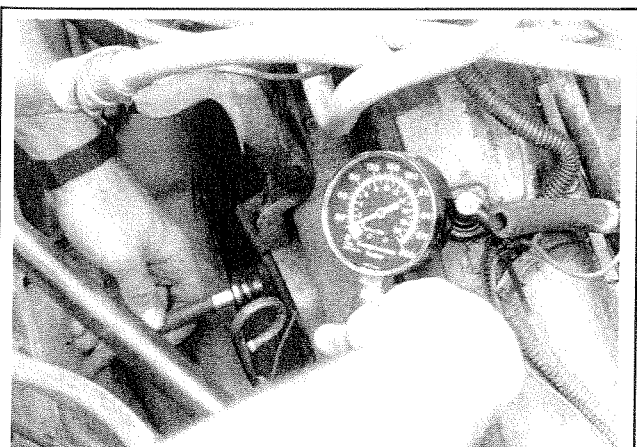
Fig. 136 A special diesel compression gauge should be used to test your engine's compression. Diesel gauges can withstand the extreme cylinder pressure developed by a diesel engine
