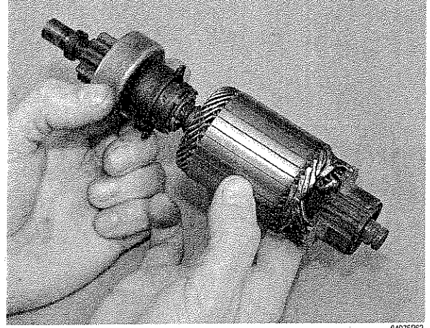
Fig. 19 This starter motor armature was destroyed from excessive engine cranking
