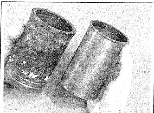
Fig. 157 Examples of a wet cylinder liner (left) and a dry liner (right) Note the corrosion on the wet liner from exposure to salt water
