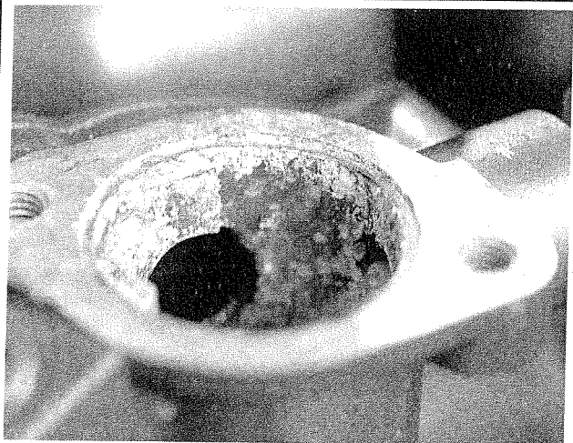
Fig. 66 Excessive corrosion in the thermostat housing may indicate problems in the header tank
