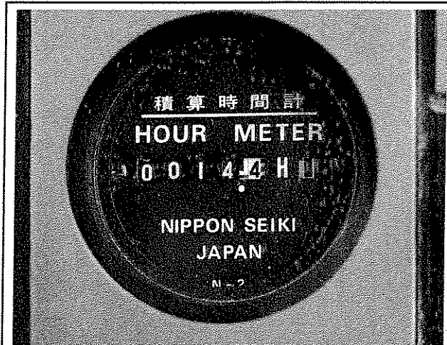
Fig. 41 Hour meters are essential for keeping track of maintenance intervals
