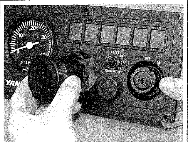
Fig. 66 . . . and pull the buzzer from the front of the panel
