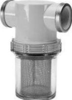
Mount the sea strainer with the provided 3/4" NPT nylon nipple directly to the intake of the 20 micron pre-filter housing. If an optional boost pump is required (refer to "Available Options and Accessories"), mount the sea strainer in a serviceable location in between the sea-cock of your choice and the boost pump.
