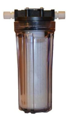
The ECHOTec post treatment element contains a mixture of minerals that returns bicarbonate alkalinity, correcting pH only enough to reach a neutral equilibrium. This dramatically reduces corrosion on metal tanks, boilers, washing machines and plumbing due to acidic product water.
