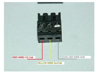
Make sure, that cables are connected as shown above. A wrong connection could damage the converter or other devices on the SeaTalk Bus.
