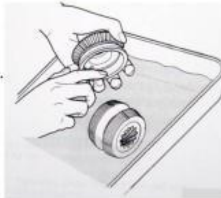
Figure 12: Step 7 Lapping Procedure For Drive Cone, Cont.
