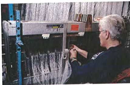
Warp yarns are still hand-threaded onto the 'sticks' that move up and down in the loom
