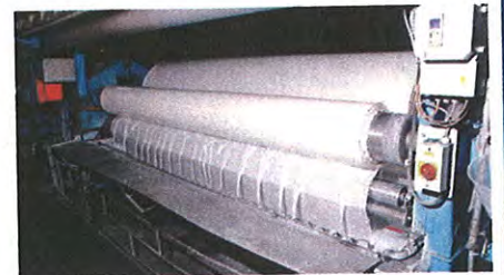
After it leaves the loom, the unfinished cloth is washed to remove lubricants
