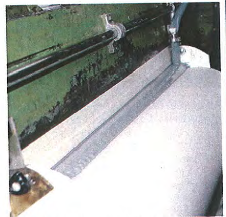
Cloth that will become protective UV strips receives its anti-ultraviolet coating
