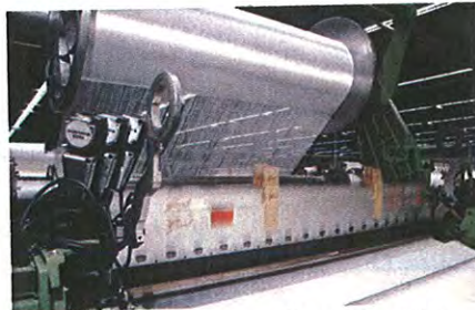
Specially adapted looms allow Dimension-Polyant to weave Dyneema into Hydra Net
