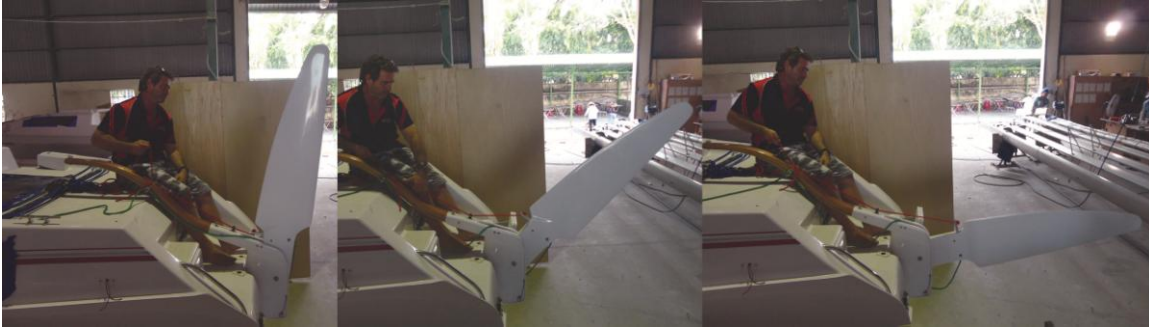
(Cruze 970 transom hung rudder being lifted up.)
