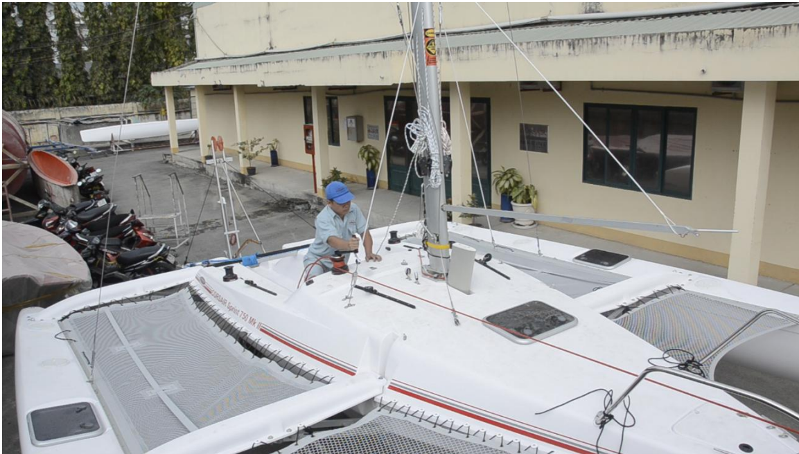
(Mast on way up and being held from going sideways by raising wires.)
