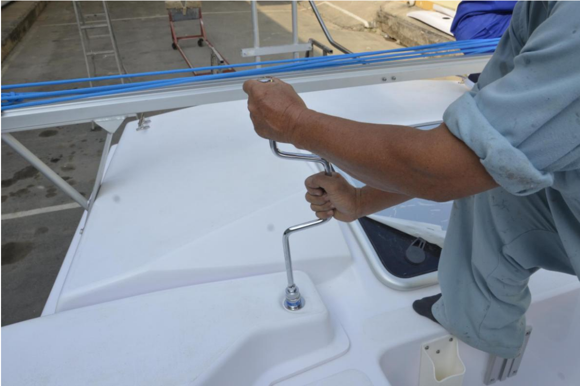
(Beam bolts must always be tightened firmly before sailing.)
