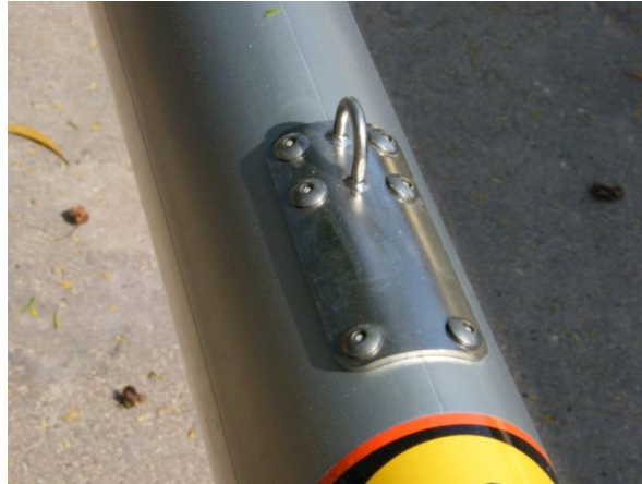
(Mast raising eye on mast.)
