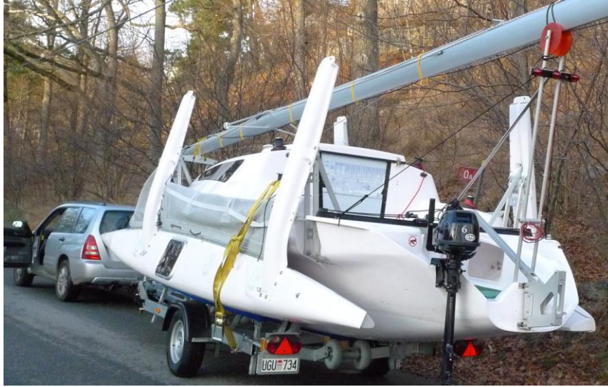
(The original prototype Dash 750, with outboard and under lugs rudder system. This type of rudder can be removed altogether for long distance trailering. Aft cockpit models all now use transom hung rudders.)
