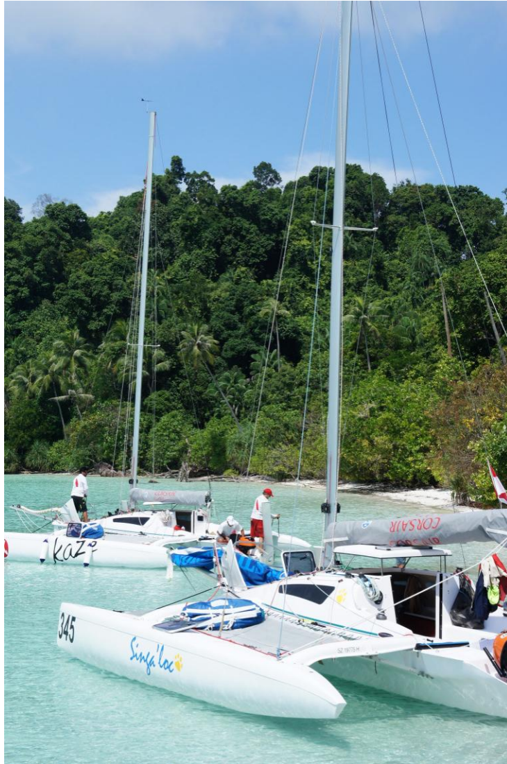
(The advantages of multihull with shallow draft can be easily seen. Sometimes you don't even need anchor. Just pull up at the nearest beach.)
