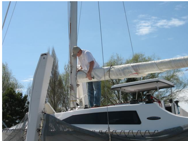
(Use the topping lift to fit/disconnect the boom.)
