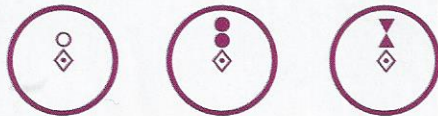
Virtual AIS beacons are shown on the chart by symbols such as these with the legend 'V-AIS'
