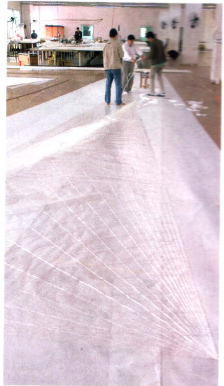
ABOVE: A 'structured tape' sail. The lines are fibres laid down on the load paths in the sail BELOW: The spinnaker loft
