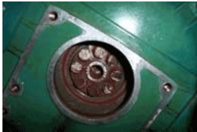
These spline shaft engages with a plate bolted to the flywheel shown in place and removed
