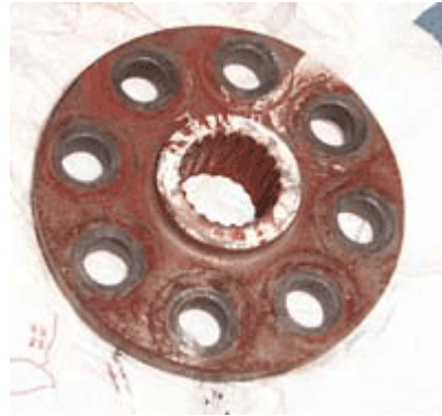
These spline shaft engages with a plate bolted to the flywheel shown in place and removed
