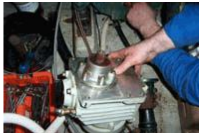
Gearbox detached from the engine and the position of the splined drive shaft
