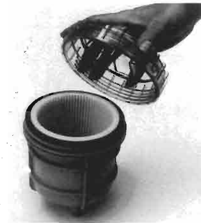
Controle koelwaterfilter. Checking raw water strainer.
