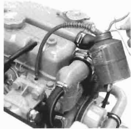
Olie inspuiten. Oil spraying.
