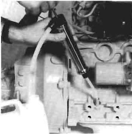
Aftappen olie. Draining the oil.
