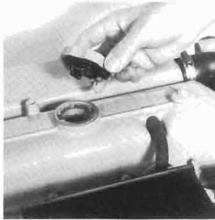
De olie vuldop. The oil filler cap.
