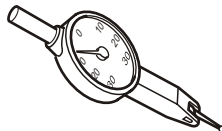
9999683 Dial indicator (short probe) Used when checking valve guides.
