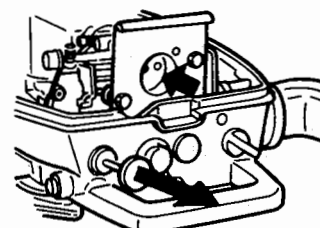
(Fig. 9-14) Checking the choke valve
