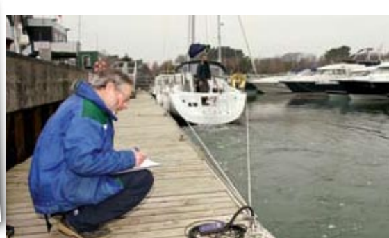
ABOVE: The load cell shackle was crucial for accurate measurement; Emrhys records a 'bollard pull'
