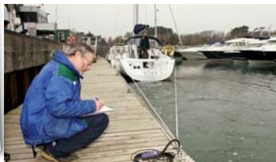
ABOVE: The load cell shackle was crucial for accurate measurement; Emrhys records a 'bollard pull'
