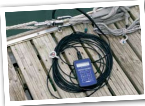
ABOVE: The load cell shackle was crucial for accurate measurement; Emrhys records a 'bollard pull'
