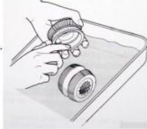
Figure 12: Step 7 Lapping Procedure For Drive Cone, Cont.
