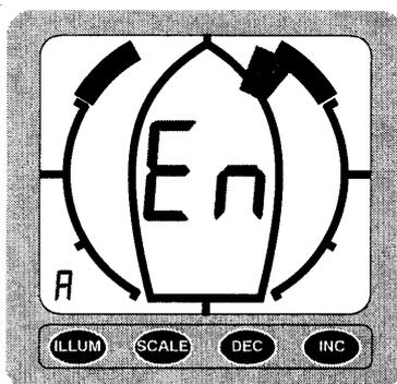
Figure 7 : mode configuration (EN)
