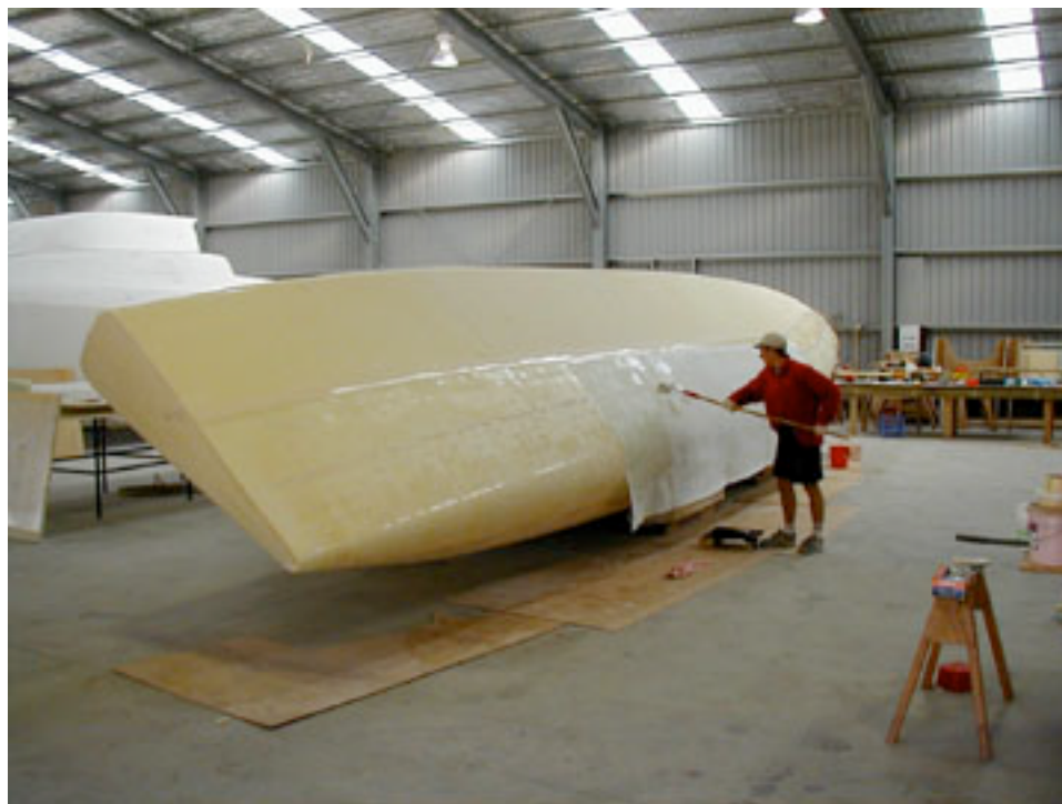
Laminating hull side of an F-41. Laminating is fairly straight forward, and once one has had some practice, it becomes relatively easy. Just don't try too big of an area at one time until familiar with the process - even very large hulls can be broken down into easy to handle small areas.
