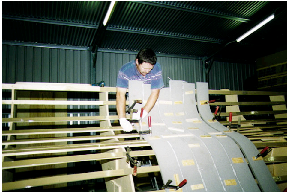
Jack Dearden starting to lay the foam strips on the hull side of his F-41. Fitting the strips is fairly straight forward, and one soon learns the various techniques and tricks required. Jack is also using some clamps to help hold in place prior to screwing.
